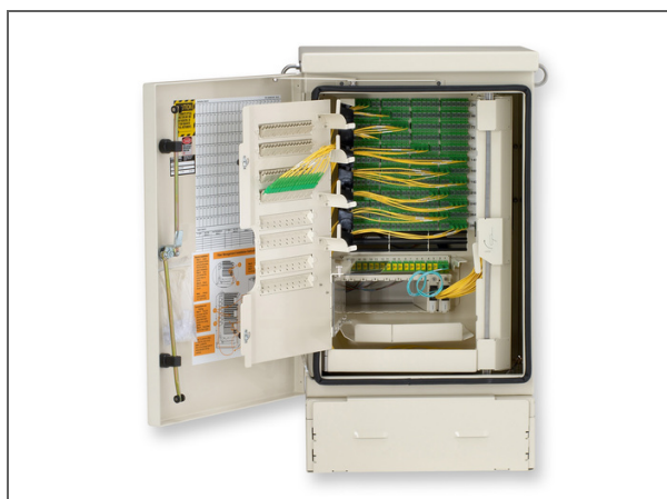
Gen III Series Outdoor Cabinet, 288 F pad-mount without toning, 48 F feeder SST-Ribbon™ cable, 1x288 F distribution ALTOS® ribbon cable, 31 m stubs, SC APC, no splitter
