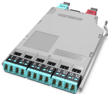
EDGE™ Solutions Tap Module, 50 µm MM (OM4), 50/50 split ratio (live/tap), 12F LC duplex ports, one pinned MTP® adapter labeled LIVE, one pinned red MTP adapter labeled TAP, enables six monitored ports, Universal Polarity
