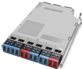
EDGE™ Solutions Tap Module, Single-mode (OS2), 70/30 split ratio (live/tap), two red LC duplex adapters labeled TAP, four blue LC duplex adapters labeled LIVE
